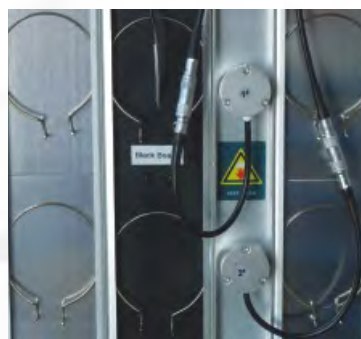
Four sensors monitor UV irradiance
