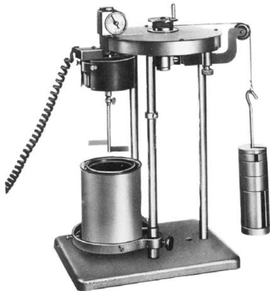
FIG. 1 Stormer Viscometer with Paddle-Type Rotor and Stroboscopic Timer
